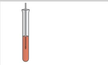
Many error-prone manual steps result in incorrect dilution ratios. A very low number of cells counted in a pre-diluted sample leads to very low accuracy with conventional analyzers.
